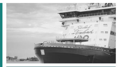
"The exterior cameras allow us to monitor the ice and the vessels we are escorting. We can use the cameras located on the stern to monitor changes in our distance to vessels that we are guiding in or out of a port. The vessel may be only a few meters behind the icebreaker or even tethered to the icebreaker if it's being towed."
