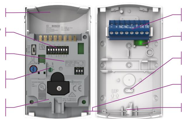
Removable, terminal block with a 45 lift-gate for easy access to the terminals
